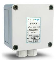
Syra IS is the module capable of making diagnosis and ON/OFF command to control the lamp. It is installed underground. Power line communication through 1.024 protocol.
